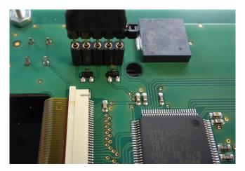
Now you have to establish a power supply connection (7 to 32VDC/max.100mA).
