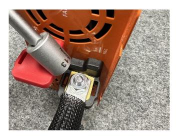
C. Connect X7:1 to positve terminal of load. Follow the recommendations of the load manufacturer.
