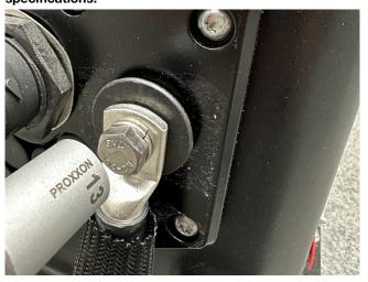
D. Connect X7:2 to negative terminal of load. Follow the recommendations of the load manufacturer.
