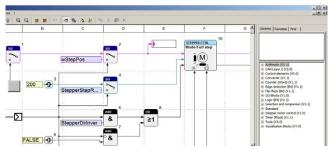
Programming the STG-700 follows using the USB port of your PC with installed miCon-L software suite and the VK-16 USB Connection Cable. The miCon-L Software supports full simulation and visualisation operation modes. miCon-L provides a variety of visualisation blocks and interactive elements to control and debug the Mini-PLC.
