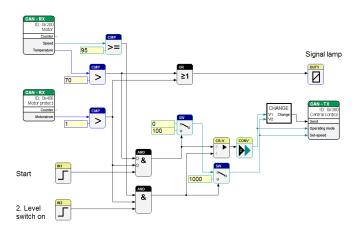
Programming the STG-570 follows using the USB port of your PC with installed miCon-L software suite and the VK-16 USB Connection Cable. The miCon-L Software supports full simulation and visualisation operation modes. miCon-L provides a variety of visualisation blocks and interactive elements to control and debug the Mini-PLC.
