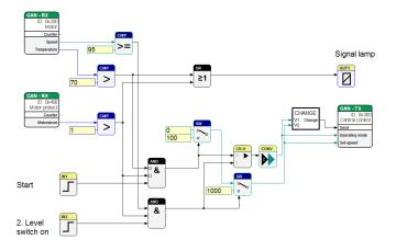
Programming the STG-550 follows using the USB port of your PC with installed miCon-L software suite and the VK-16 USB Connection Cable. The miCon-L Software supports full simulation and visualisation operation modes. miCon-L provides a variety of visualisation blocks and interactive elements to control and debug the Mini-PLC.
