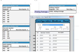
Programming the STG-580 follows using the USB port of your PC with installed miCon-L software suite and the VK-16 USB Connection Cable. The miCon-L Software supports full simulation and visualisation operation modes. miCon-L provides a variety of visualisation blocks and interactive elements to control and debug the Mini-PLC.
