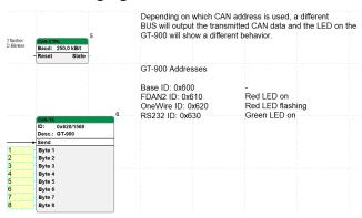
This is an overview of the miCon-L program. The CAN ID can be changed to use the corresponding communication interface on the GT-900.
