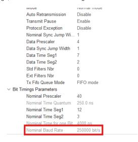
The FDCAN baudrate is changed by adjusting the "Nominal Prescaler". Changing it to ,20' will double the baudrate.
