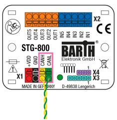
There is no termination resistor integrated in the lococube®. Please add a 120R resistor at both ends (2) for correct CAN bus termination.
