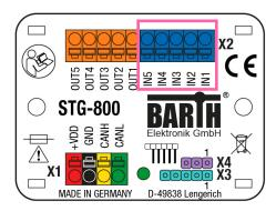
Due to the pull-down resistors integrated in the lococube® any switch (NO/NC) can simply be connected between the positive supply (VDD) and the desired input. The 10-pole connector named X2 contains the inputs of the lococube®. While IN4 and IN5 are pure digital inputs, IN1 to IN3 provide both digital or analog (0-30V) functionality. The voltage range for all inputs may not exceed 32 VDC. All inputs refer to GND.
