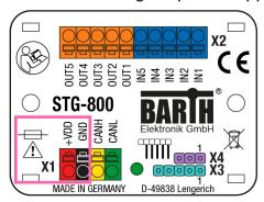
The lococube® features an outstanding wide supply voltage range from 7 to 32 VDC at lowest current consumption. So the lococube® can be integrated within battery supplied 12V or 24V DC systems (cars, trucks, battery powered cars, forklifts and digger, for example).
