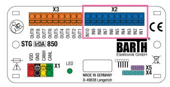
Due to the pull-down resistors integrated in the lococube® any switch (NO/NC) can simply be connected between the positive supply (VDD) and the desired input. The 10-pole connector named X2 contains the inputs of the lococube®. While IN7 to IN10 are pure digital inputs, IN1 to IN6 provide both digital or analog (0-30V) functionality. The voltage range for all inputs may not exceed 32 VDC. All inputs refer to GND.
