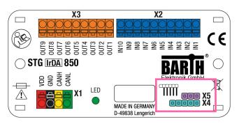
If you choose the Open Source Programming Option, use the X4 connector for programming and debugging via the Connection Cable VK-35 (BARTH® Art. No. 0091-0035). In this case the X5 connector can be used as TTL232 UART interface within your application.
