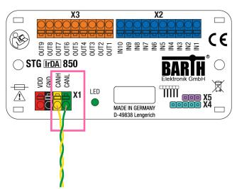
There is no termination resistor integrated in the lococube®. Please add a 120R resistor at both ends (2) for correct CAN bus termination.
