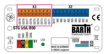
The 9-pole connector X3 contains the digital outputs of the lococube®. While OUT1 to OUT8 are overload-protected highside switches, OUT9 is carried out as lowside switch with PWM capability without short circuit protection.
