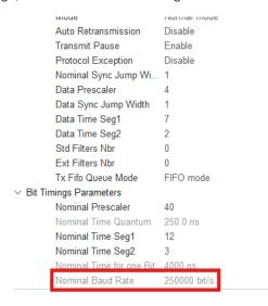
The FDCAN baudrate is changed by adjusting the "Nominal Prescaler". Changing it to ,20' will double the baudrate.
