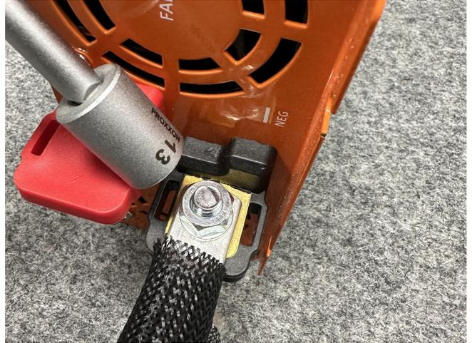
**C. Connect X7:1 to positive terminal of load. Follow the recommendations of the load manufacturer.**
