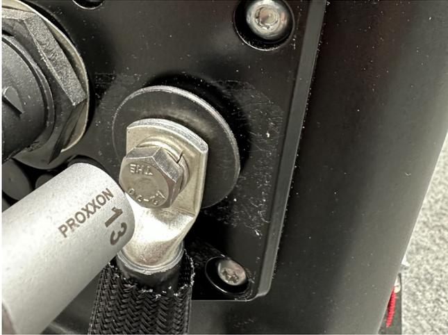
**D. Connect X7:2 to negative terminal of load. Follow the recommendations of the load manufacturer.**
