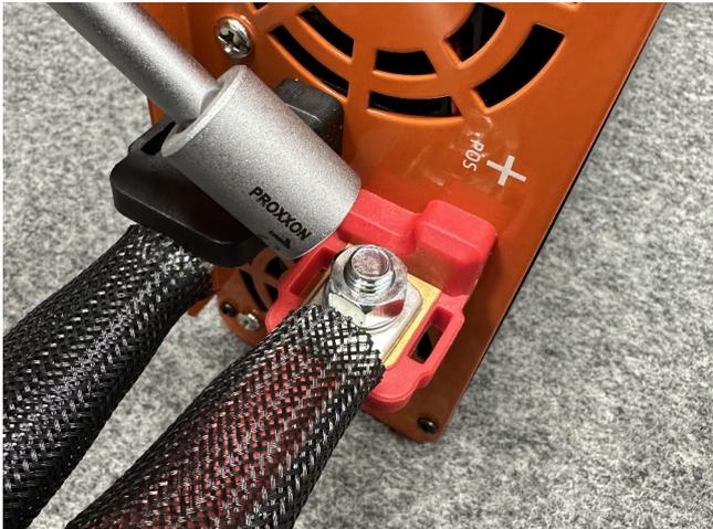
**E. Connect X5:1 to positive terminal of the charger. Use hardware supplied with your battery. Torque to charger specifications.**
