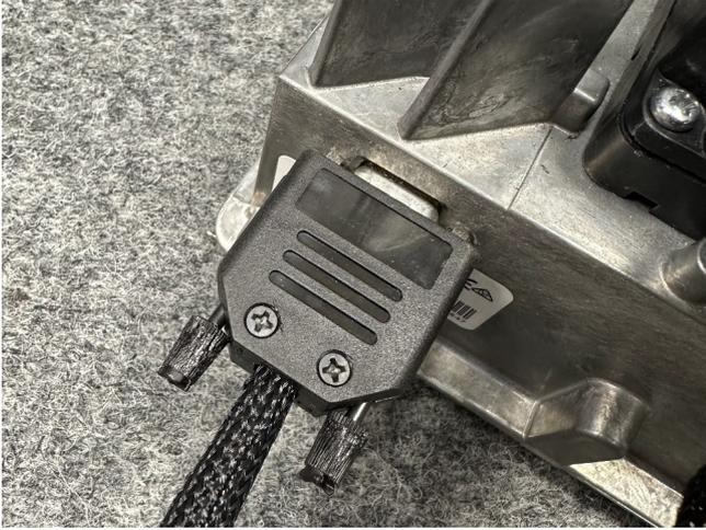
**F. Connect X1 to battery signal. Turn clockwise until endpoint is reached.**
