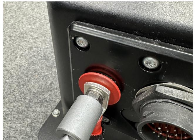
**B. Connect X2:2 to the negative battery terminal. Use hardware supplied with your battery. Torque to battery specifications.**
